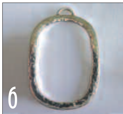
{Photo 4} Referring to chosen stone for size, forge square bar stock into an oval for outer frame. Solder join with hard solder.
